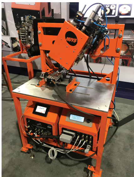
Fig. 5 — Moveable and automated ESD unit. (Courtesy of the National Research Council.)
