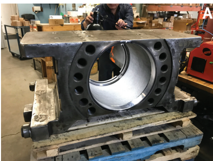
Fig. 1 — A — Steel mill chock bearing; B — close-up of chock bearing. (Courtesy of Arcelor Mittal.)
