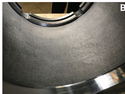
Fig. 1 — A — Steel mill chock bearing; B — close-up of chock bearing. (Courtesy of Arcelor Mittal.)
