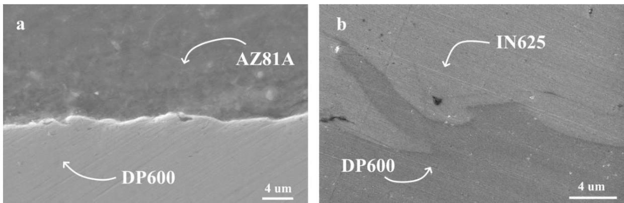
**Figure 3. a) AZ81A and b) IN625 ESD coatings on DP600 sheets prior to RSW [12]**
