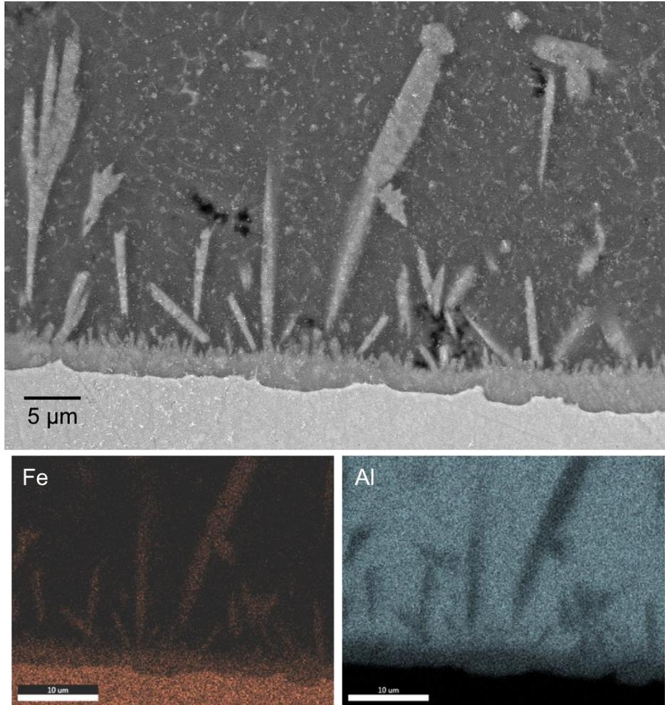
Figure 2. SEM image of an IMC at an AA5052-DP600 interface formed during RSW when no interlayer is used, as well as EDX images showing composition distribution.
