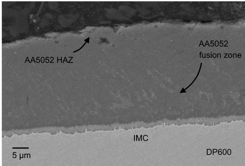
**Figure 5. SEM image of failed tensile lap shear-tested sample welded with an AZ81A interlayer**
