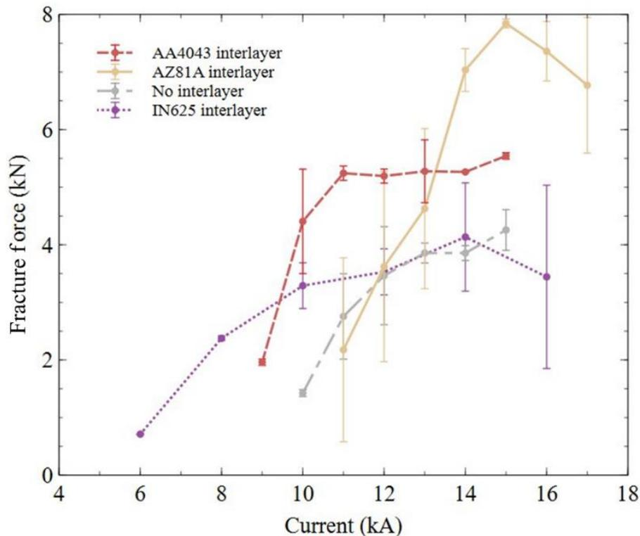
**Figure 4. Lap-shear testing between AA5052 and DP600 using different interlayer materials. Data from [11], [12]**
