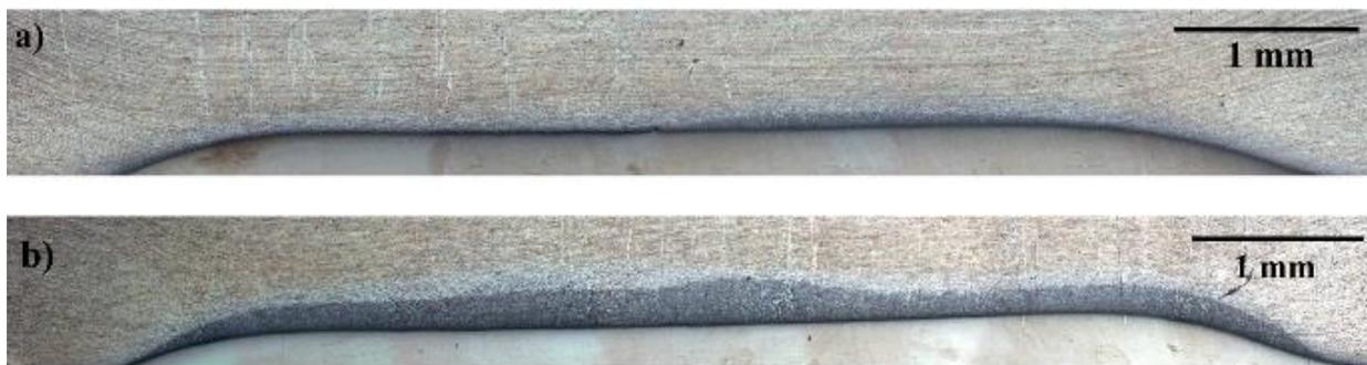
**Figure 6. Fusion zone comparison in AZ81A interlayer samples welded with (a) 13 kA, (b) 14 kA [12]**
