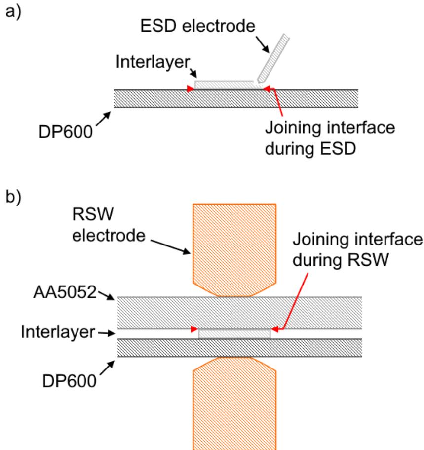
**Figure 1. Schematic of a) interlayer application on DP600 using ESD and b) Resistance spot welding of AA5052 to DP600 with an interlayer**
