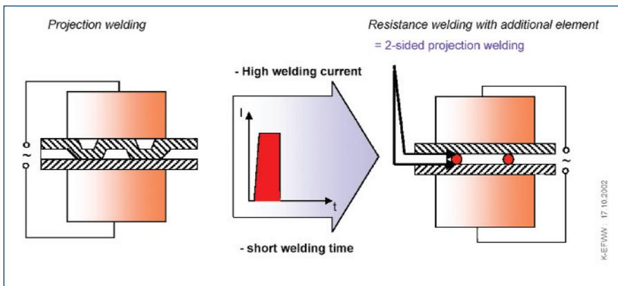
Fig. 4 — Illustrations of Volkswagen's patents for Resistance Welding with Additional Elements.
