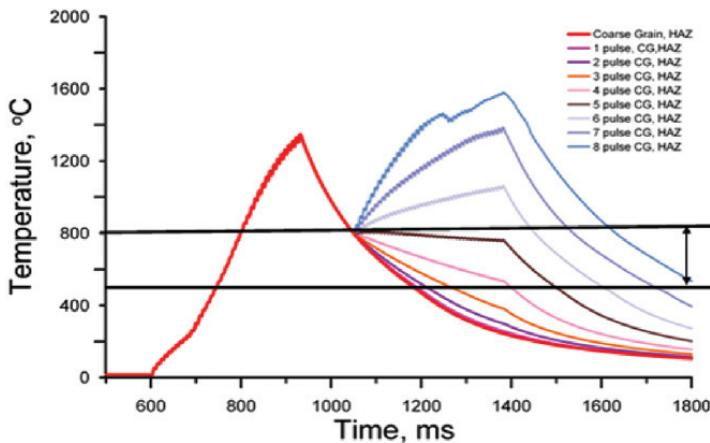
Fig. 11 — Variations in the length of a postweld tempering pulse of a weld are graphed for peak temperature and cooling rate.
