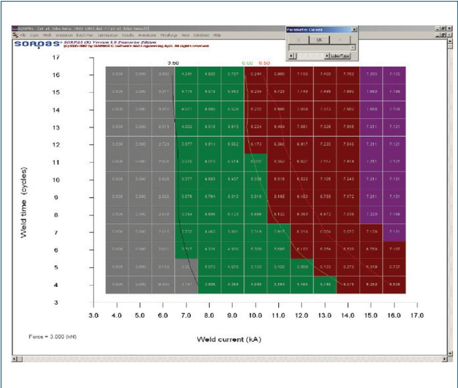
Fig. 12 — Weldability lobe diagram.
