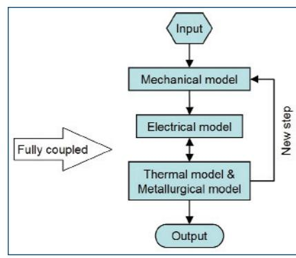
Fig. 2 — The coupling of numerical models.
