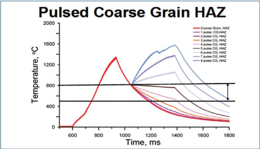
Fig. 11 — Variations in the length of a postweld tempering pulse of a weld are graphed for peak temperature and cooling rate.
