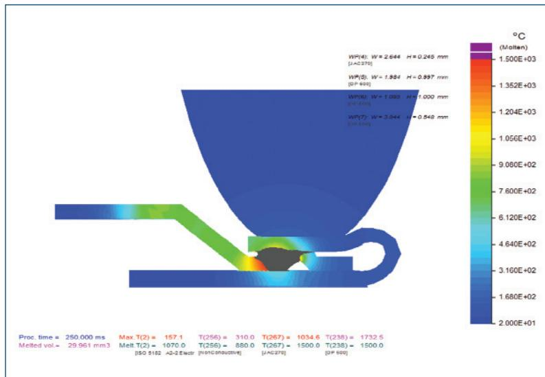
Fig. 7 — A finished simulation illustrating a specific combination of welding parameters and projection designs.
