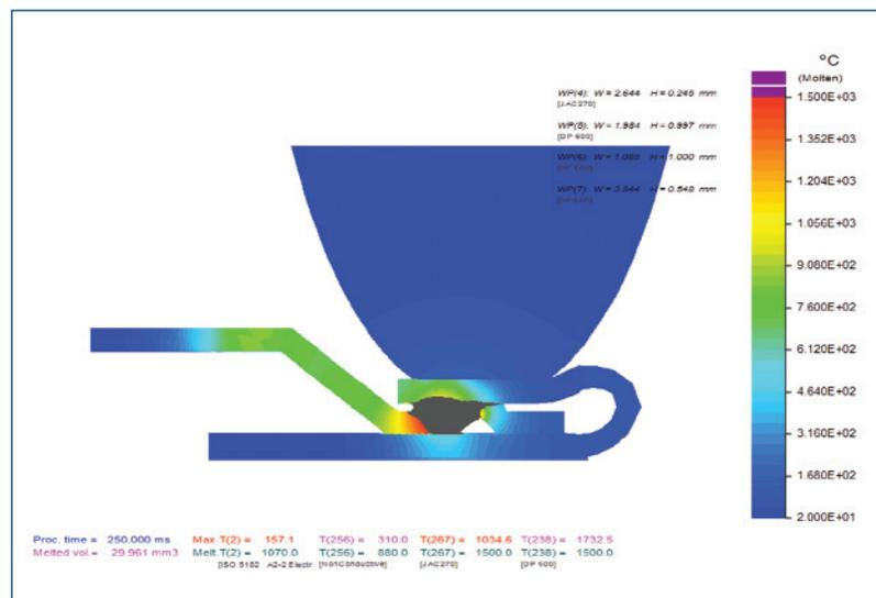
Fig. 7 — A finished simulation illustrating a specific combination of welding parameters and projection designs.
