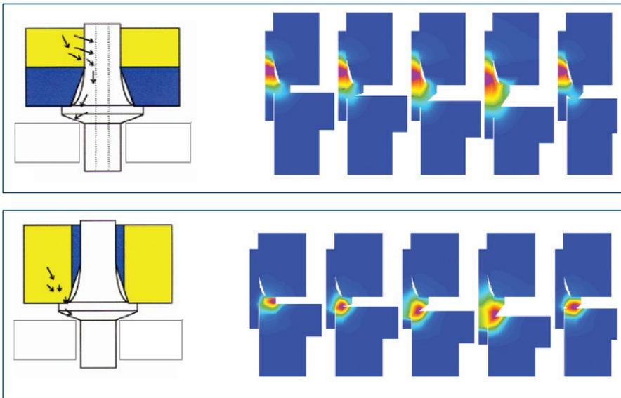
Fig. 5 — Example of using different insulation designs (left) to generate different welding characteristics.
