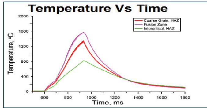
Fig. 9 — Graphs indicating time and temperature during the welding of specific sites, or nodes, of the weldment (see Fig. 8).
