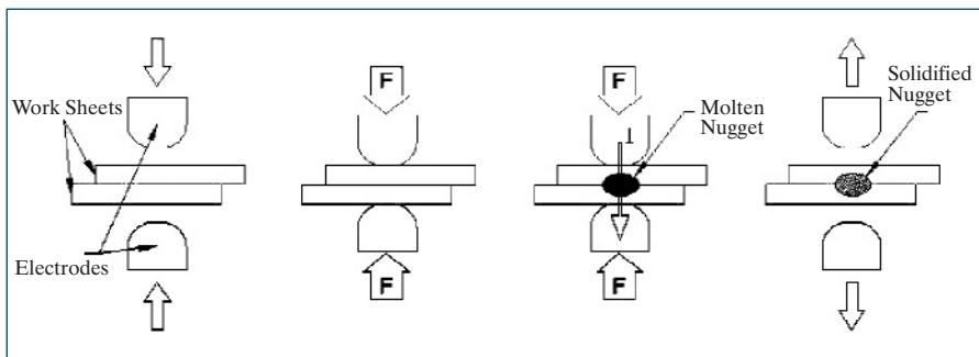
Fig. 1 — The basics of the resistance welding process.
