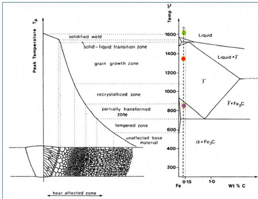
Fig. 10 — A published constant cooling diagram indicating the peak temperatures from Figs. 8 and 9.
