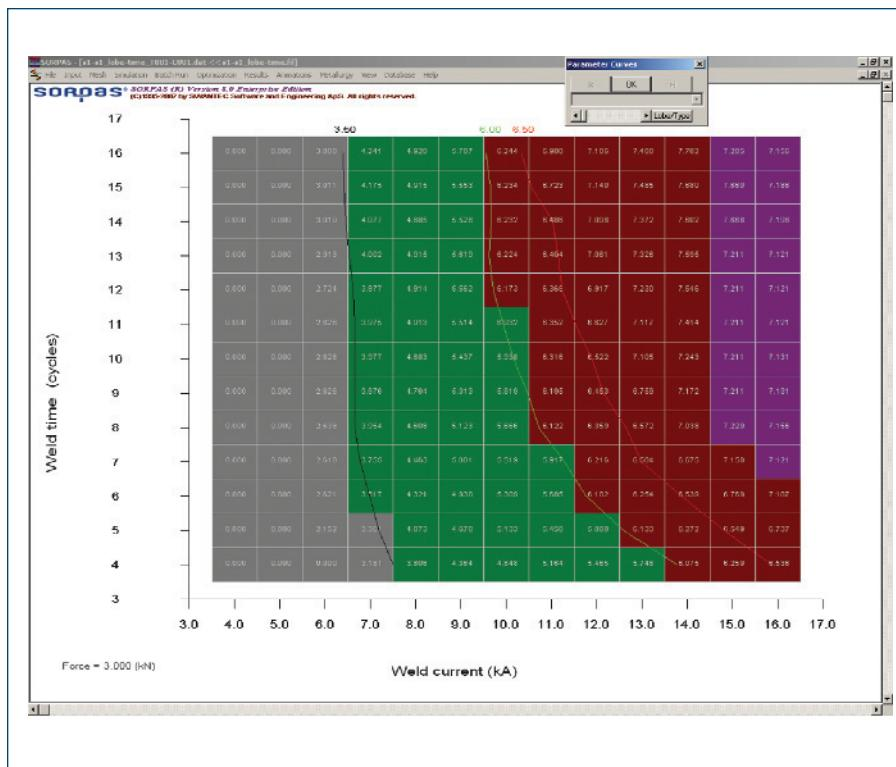
Fig. 12 — Weldability lobe diagram.
