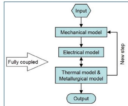
Fig. 2 — The coupling of numerical models.
