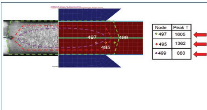
Fig. 8 — A metallographic photograph and a simulation showing peak temperatures in different regions of the weld and HAZ.
