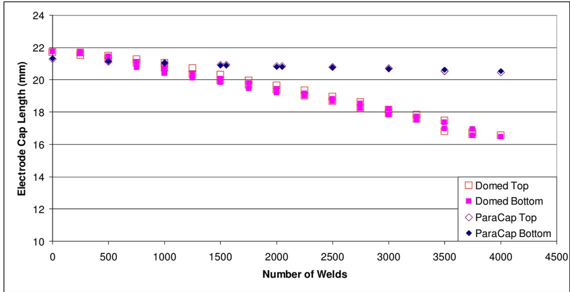
Fig 16: Electrode length measurements at each dressing interval for Production Test Run Two.
