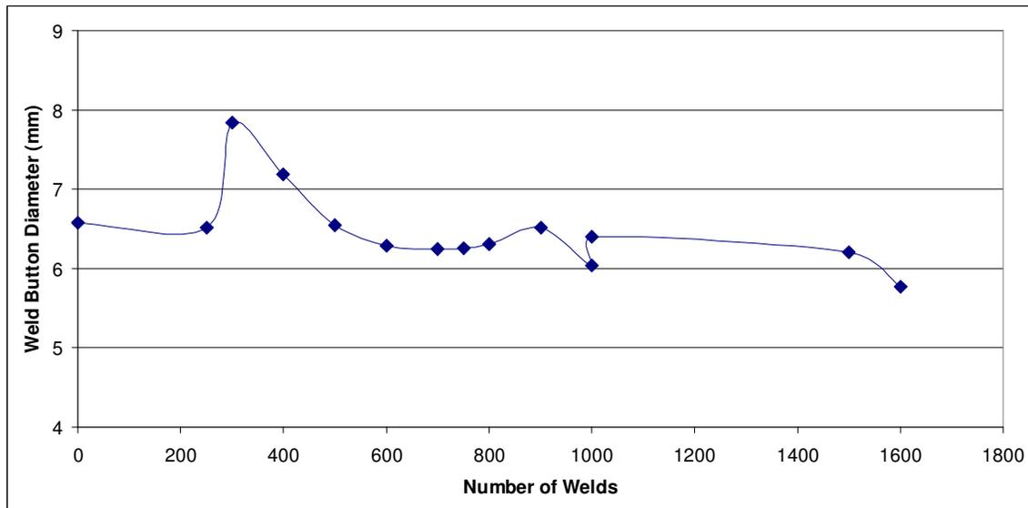
Fig 14: Weld button size vs. number of welds for production test one. Dressing was performed whenever button size dropped below 6.0mm.
