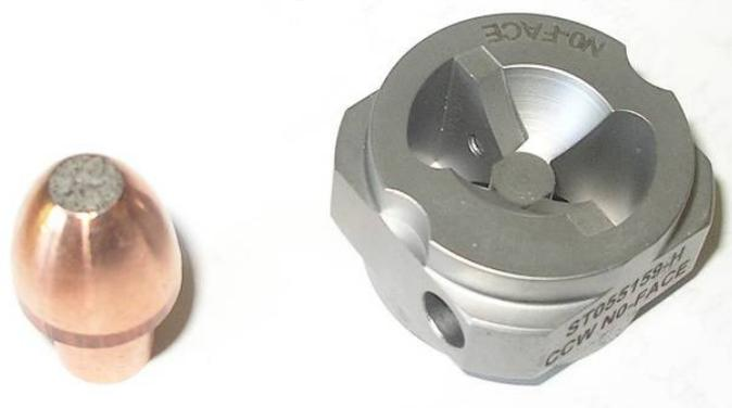
Fig 5:, A parabolic male cap and a side dressing blade.,
