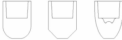
*Fig 1: A typical dome (FB), a truncated (FE) and a parabolic (ParaCap™) style electrode*
