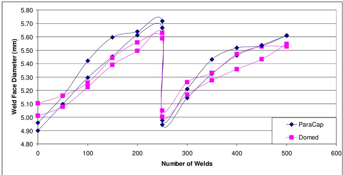
Fig 9: Tip growth for parabolic and domed electrodes
