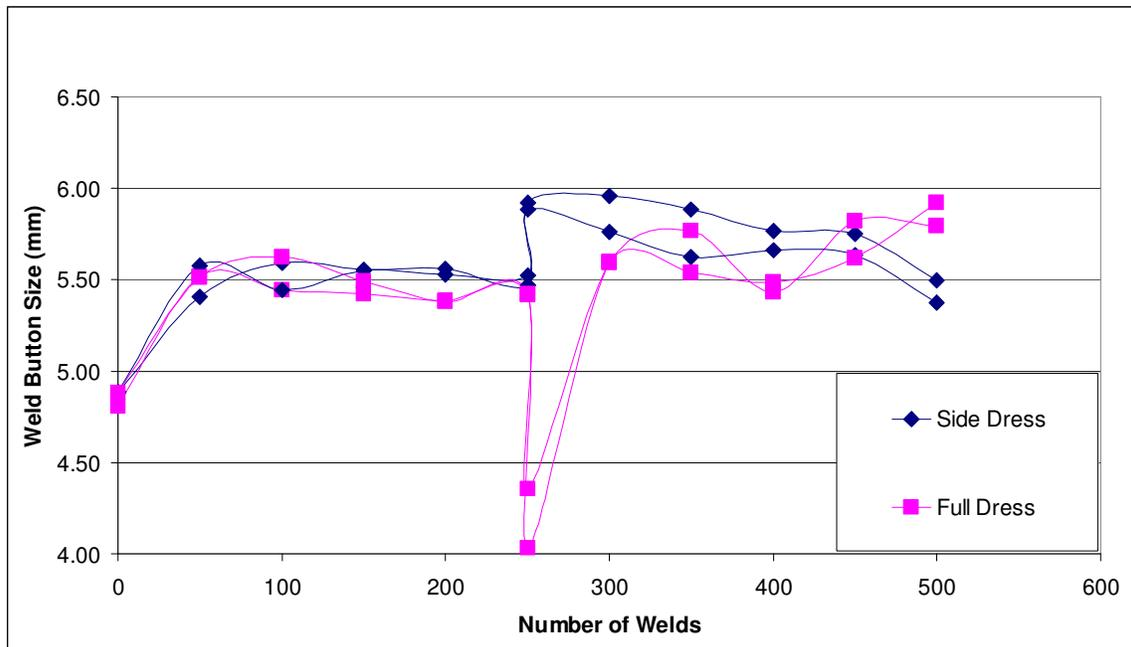
Fig 11: Weld button size increase after side dressing only compared to sudden weld size drop after full dress. Dressing operation at 250 welds
