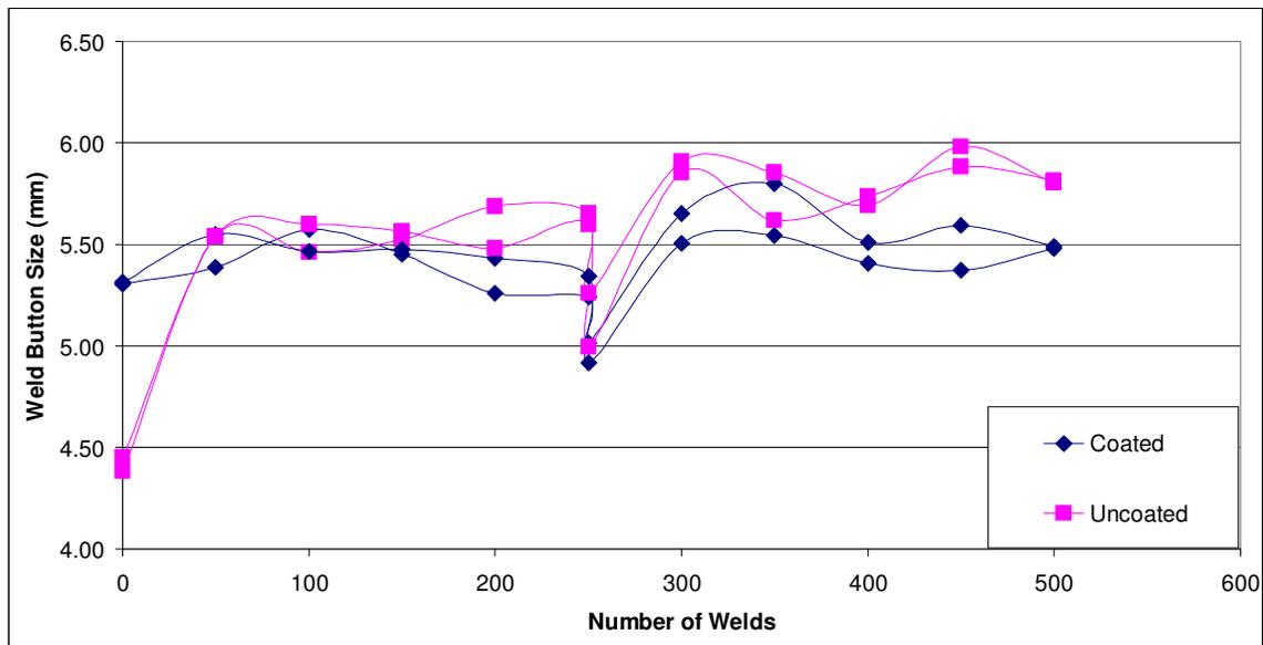
Fig 8: Weld peel button size vs. number of welds for uncoated and coated electrodes
