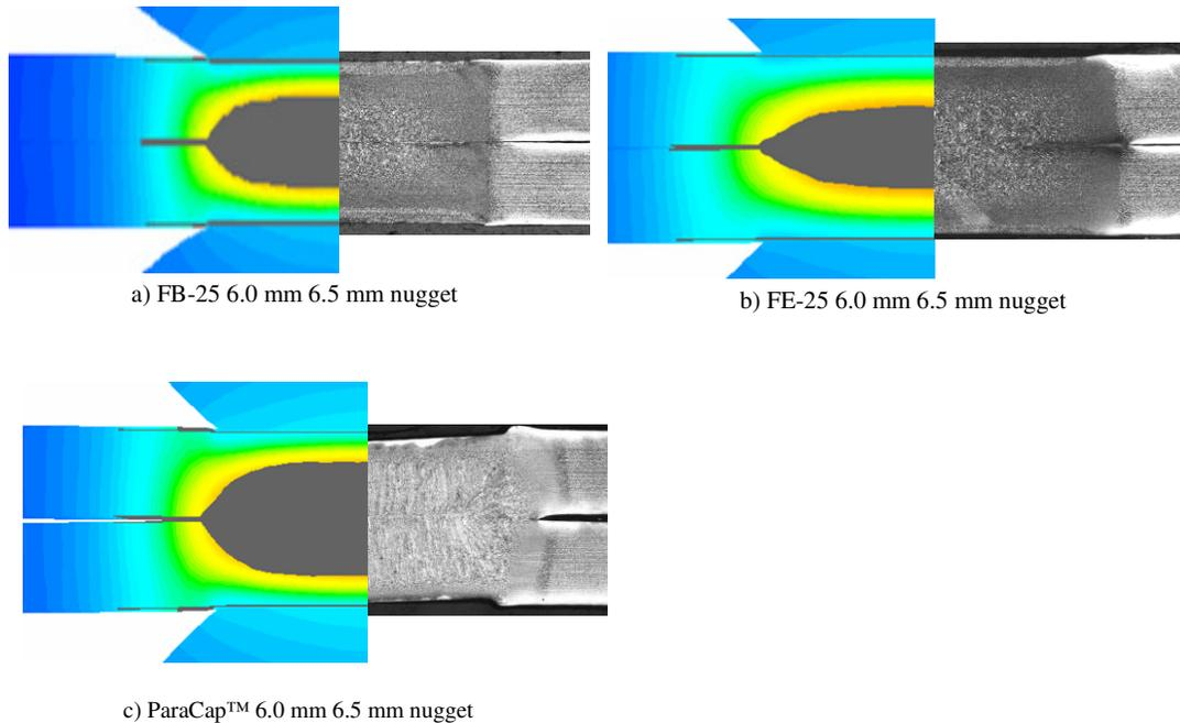
*Fig 2: Sorpas®[17] simulations and matching micrographs of welds achieved with different geometries using similar welding schedules. [7]*
