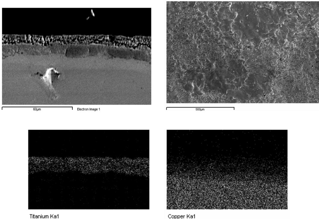
*Fig 3: SEM surface and cross section of new multilayer coating (Tricoat™). EDS elemental mapping of Ti, Ni, and Cu are shown to exhibit coating thickness and consistency.*
