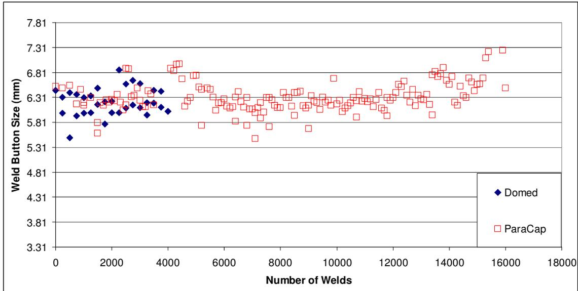
Fig 18: Weld button size vs. number of welds for production test three. ParaCap™ results are compared with domed electrode results from production test two
