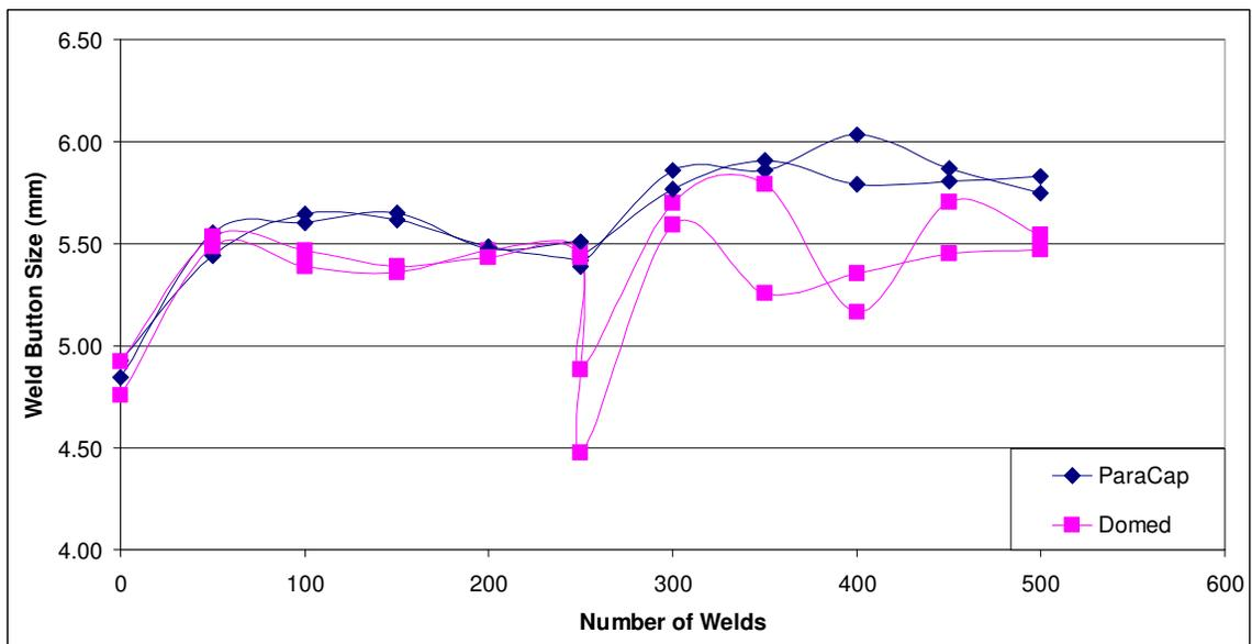
Fig 10: Weld button size for parabolic and domed electrodes
