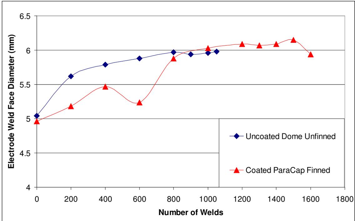
Fig 13: Weld face diameter growth curves for improved and conventional electrode designs
