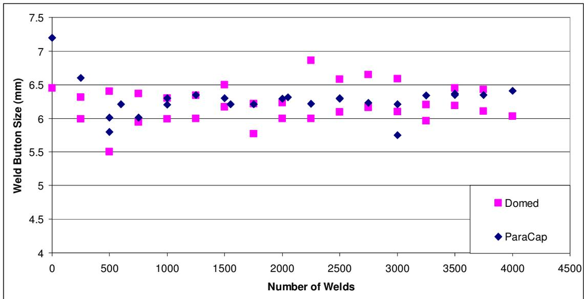
Fig 15: Weld button size vs. number of welds for production test two with dressing every 250 welds for domed electrode, and every 500 welds for ParaCap™.
