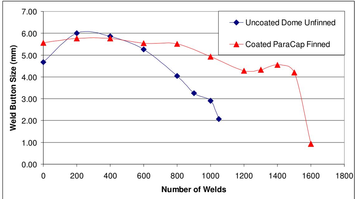
Fig 12: Electrode life test results for Improved electrode design (coated, parabolic, finned and side dressed) compared to conventional (uncoated, domed, unfinned and fully dressed) electrode design.
