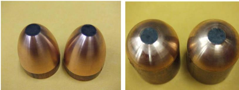
*Fig 6: Images of caps to be used in testing. ParaCaps™ at left, domed at right.*
