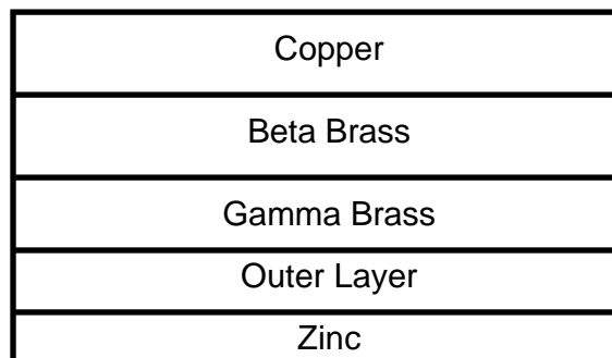
Figure 2.9: Typical electrode alloy layer schematic [5]
