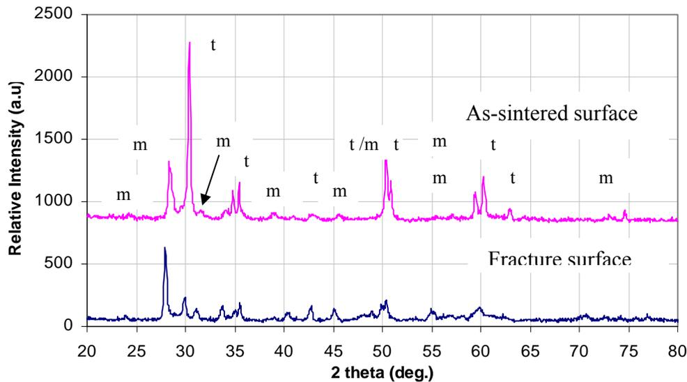
Figure 2 X-ray diffraction patterns of FMM-2 Ce-PSZ ceramics. t and m stand for tetragonal and monoclinic  $ZrO_2$  phases respectively
