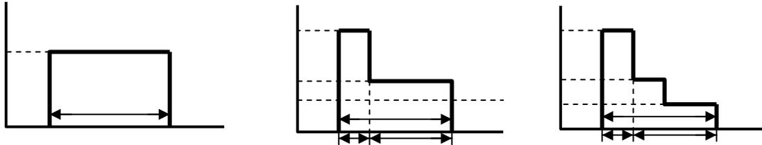
*Figure 2. Types of current inputs tested, from left to right, a single pulse weld, a 2-pulse weld and a 3-pulse weld.*
