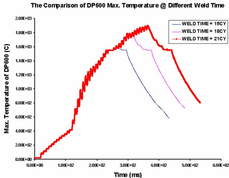
*Figure 3. Maximum temperature of 1-pulse welding with different weld times simulated by SORPAS® software.*
