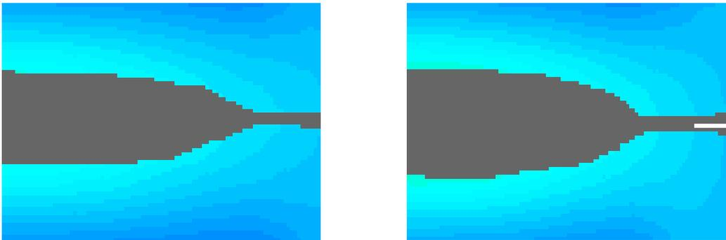
*Figure 1. Nuggets simulated by SORPAS® software, using a 2-pulse current with the left diagram illustrating a 2 cycle first pulse and the right a 5 cycle first pulse.*
