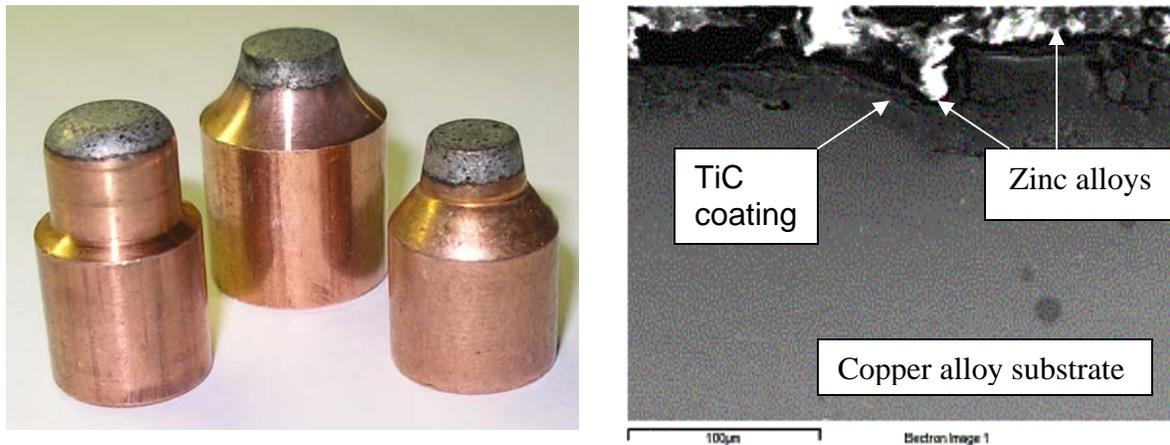
*Figure 5. Left are titanium carbide coated electrodes (TiCap™) and, right, a SEM cross section of a used TiCap™ showing the coating's effectiveness of retarding molten zinc alloys' attempt to migrate, once vapourized in welding, into the copper alloy electrode.*
