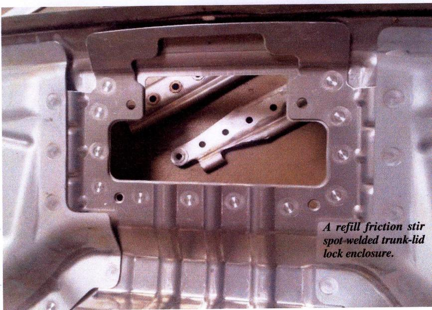
*A refill friction stir spot-welded trunk-lid lock enclosure.*
