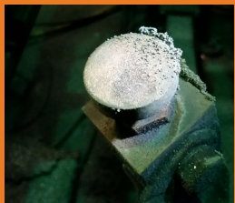
Worn Traditional Ground Block
