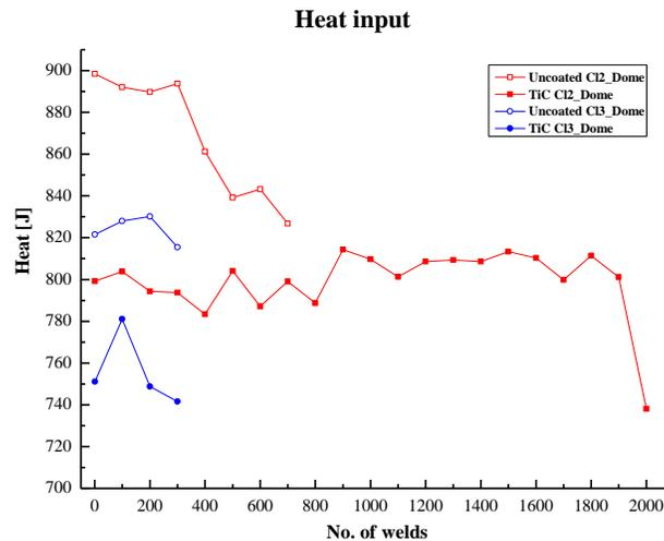
**Figure 10. Heat input of Class 2 and Class 3 dome electrodes**
