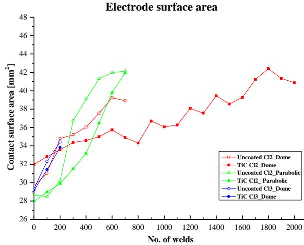
Figure 7. Changing of electrode surface area
