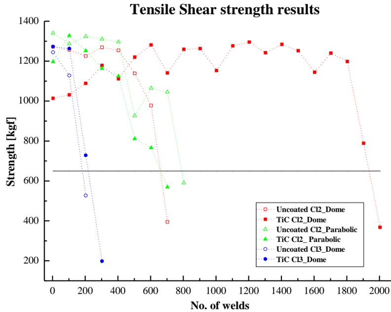
Figure 3. Tensile shear strength results
