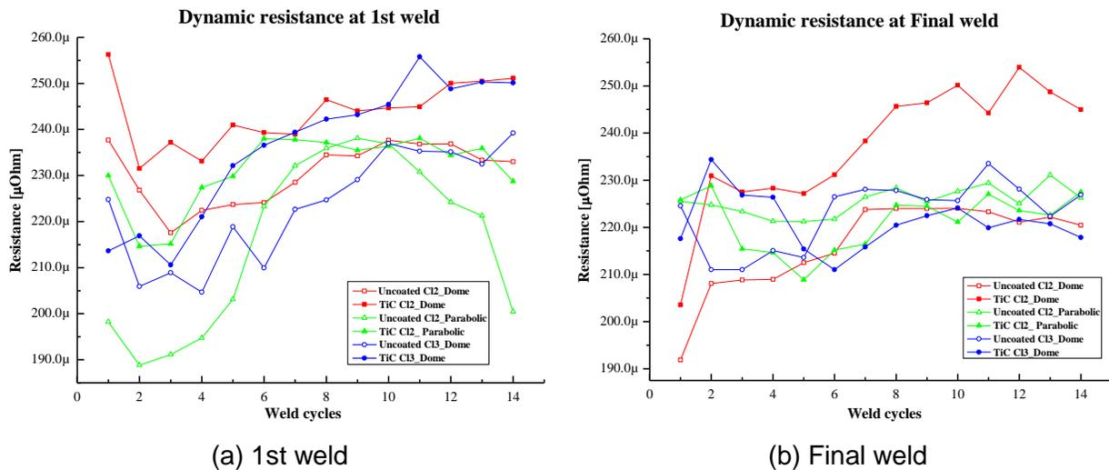
Figure 6. Dynamic resistance curves at (a) 1st weld and (b) Final welds
