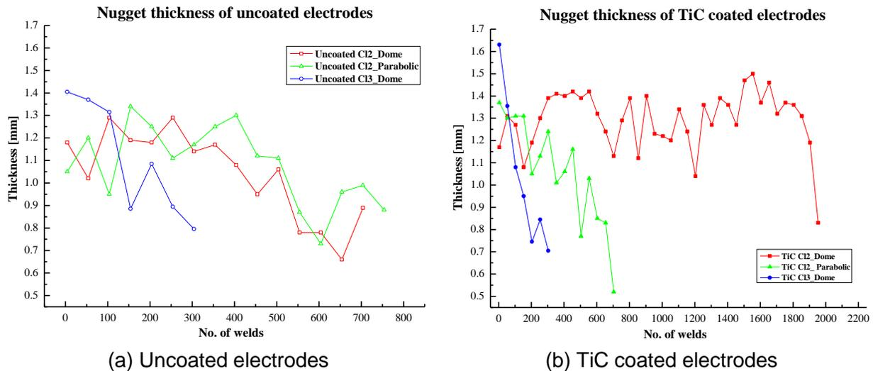
Figure 9. Nugget thickness, (a) Uncoated electrodes and (b) TiC coated electrodes
