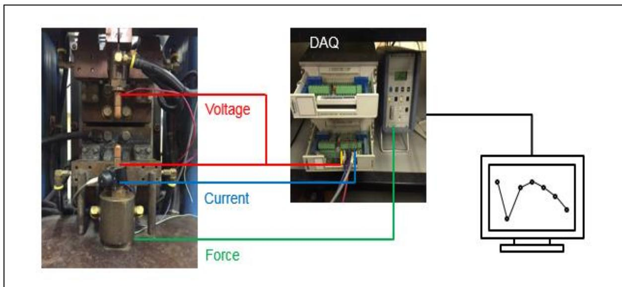
**Figure 1. Schematic of resistance spot welding system**
