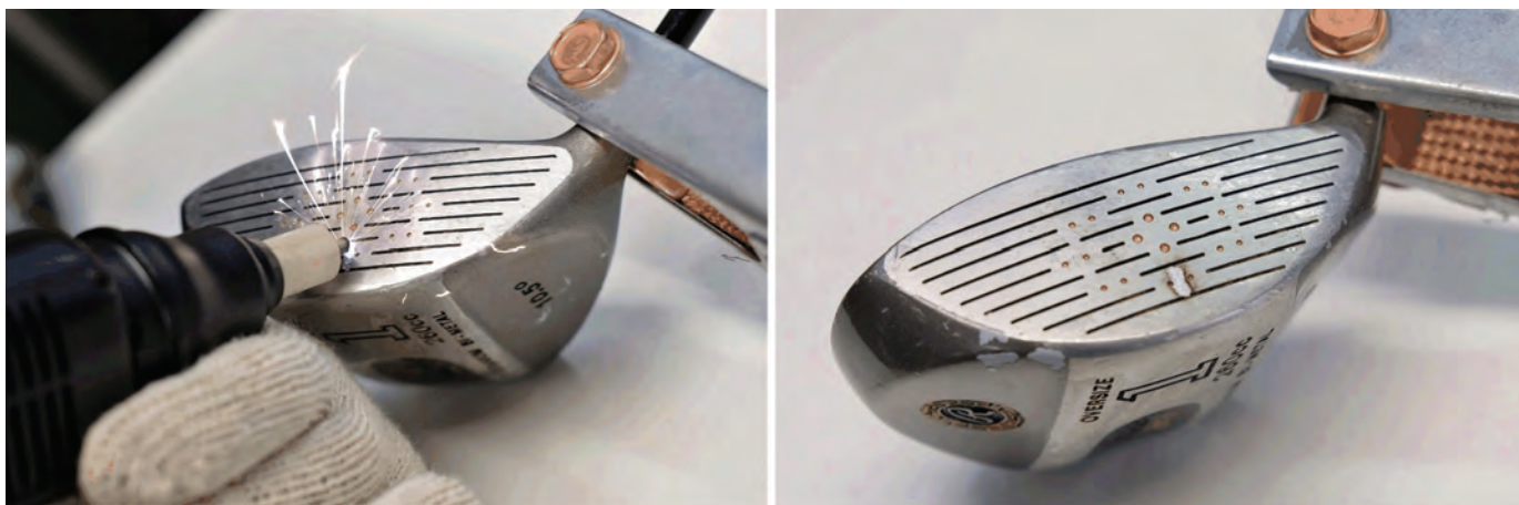
Fig. 2 — LEW repair of a titanium alloy golf club. (Photo courtesy of Huys Industries.)
