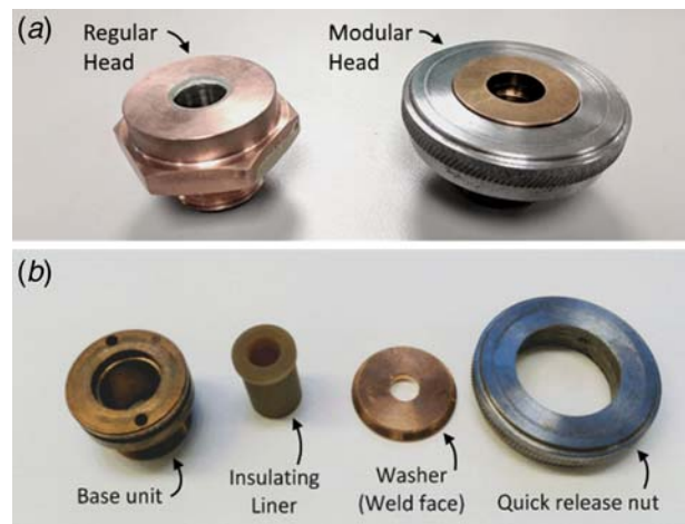
Fig. 2 Bottom electrodes showing (a) regular head and assembled modular head and (b) disassembled modular head
