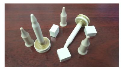
Our ceramic pins are made of hard, stabilized zirconium oxide or silicon nitrate, which provide longer life than steel pins with no risk of electrical shorting. Due to the high hardness and manufacturing process for the ceramic, all parts are finished to specification by diamond grinding. This does increase the lead time and cost for each pin.
